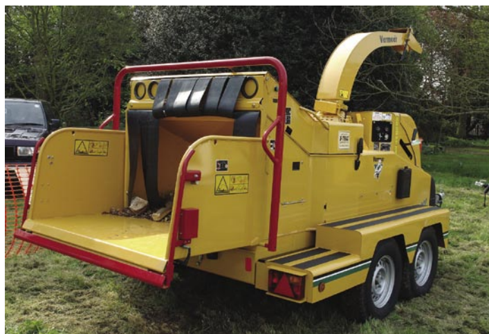
(Left) Carlton's 9 inch 1790 which was launched last year. (Right) The Vermeer BC1400XL from B-Trac has an in-feed opening of 15" x 20".
