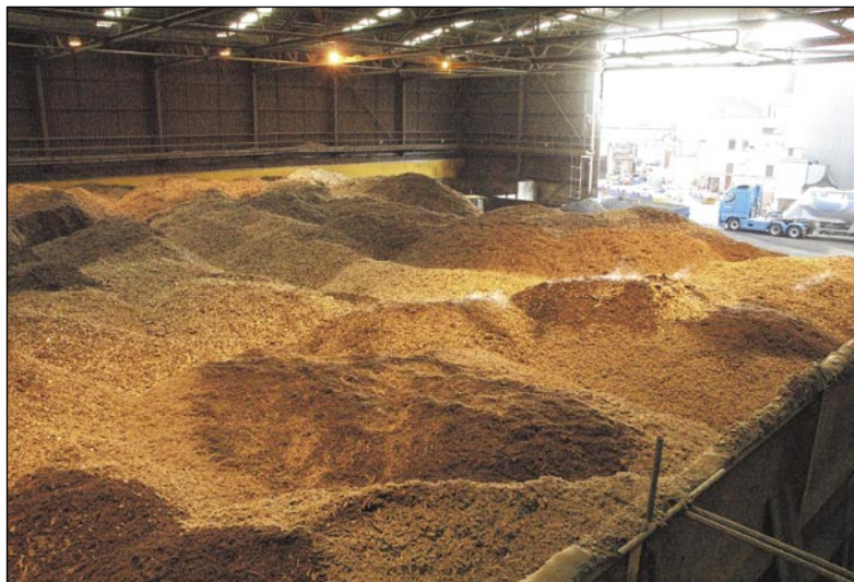
(Left) Piles of biomass steam as the water evaporates away. This store holds 20,000 square foot of biomass, which Slough Heat and Power will burn in a day. At the back of the image, just by the left of the opening, the tops of two coal piles can be seen. (Right) A Volvo shovel loader with a 7 cubic metre scoop in the fuel store, loading a mix of biomass chips with waste wood into the moving floor so it can begin its journey towards the biomass boiler.
