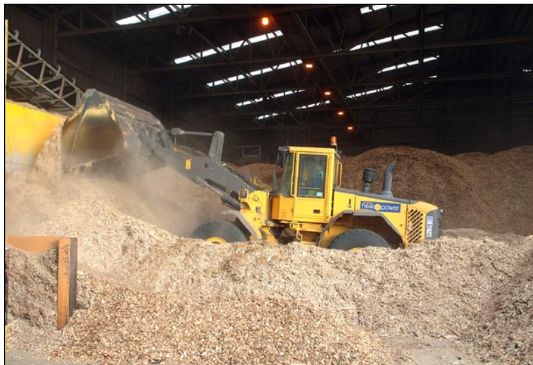
(Left) Piles of biomass steam as the water evaporates away. This store holds 20,000 square foot of biomass, which Slough Heat and Power will burn in a day. At the back of the image, just by the left of the opening, the tops of two coal piles can be seen. (Right) A Volvo shovel loader with a 7 cubic metre scoop in the fuel store, loading a mix of biomass chips with waste wood into the moving floor so it can begin its journey towards the biomass boiler.
