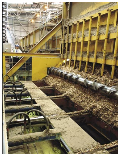
(Left) The biomass gets loaded onto the walking floor infeed system, it comes through the wall and is mixed before dropping through onto a vibratory feeder to convey its way up to the boilers. (Right) Piles of biomass steam away before they are scooped onto the vibratory feeder (at base of yellow wall in middle of image) to begin their ten-minute journey starting at the base of this conveyor belt.
