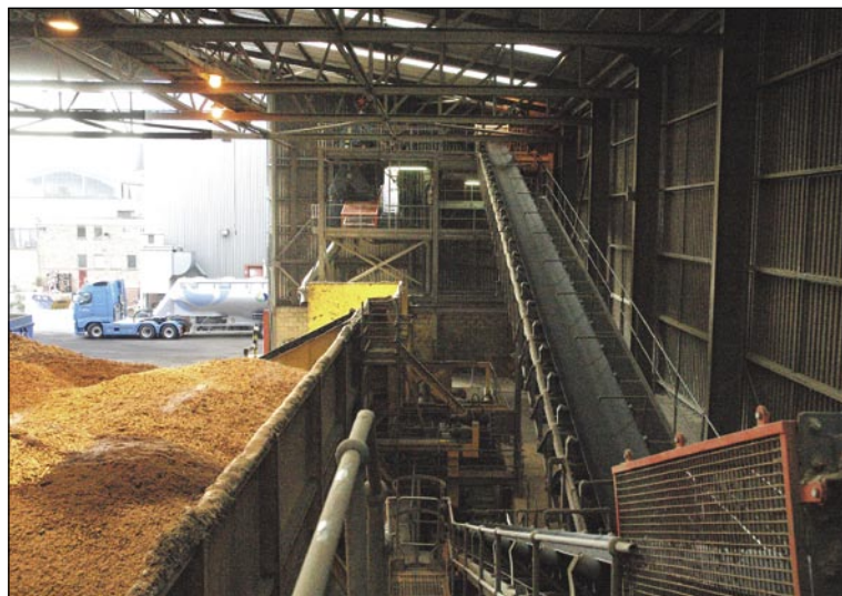
(Left) The biomass gets loaded onto the walking floor infeed system, it comes through the wall and is mixed before dropping through onto a vibratory feeder to convey its way up to the boilers. (Right) Piles of biomass steam away before they are scooped onto the vibratory feeder (at base of yellow wall in middle of image) to begin their ten-minute journey starting at the base of this conveyor belt.
