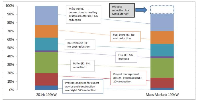
Figure 3: 199kW Cost Reduction Forecast
