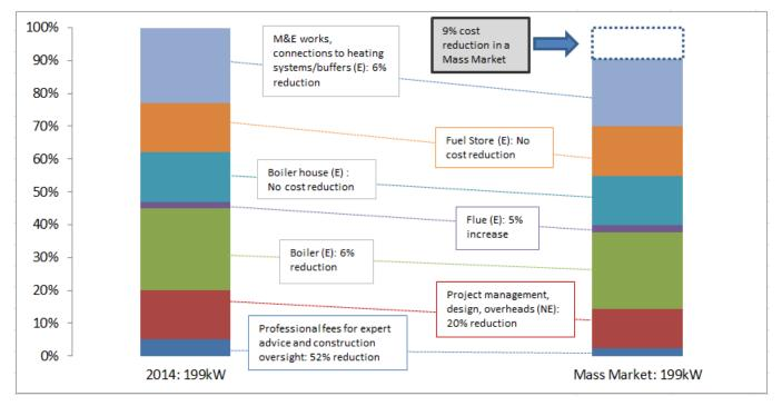
Figure 1: Cost reductions for a 199kW boiler
